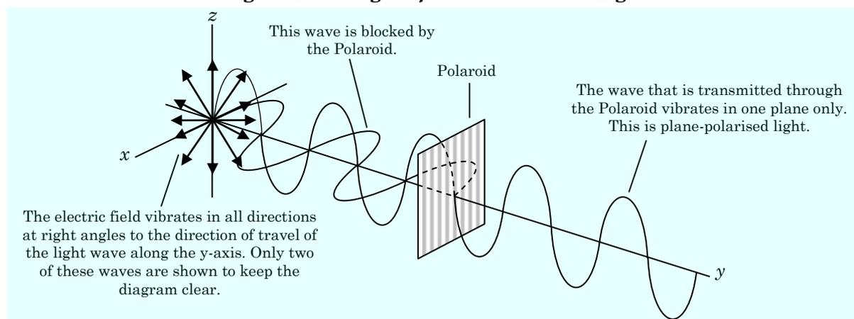
Figure 20.5 shows what happens if we shine the plane-polarised light onto a second Polaroid film. This second filter is called the analyser. If the two Polaroid films (polariser and analyser) have their polarising axis aligned, the maximum amount of plane-polarised light can pass through the analyser (Figure 20.5 (a)). If the analyser is now twisted through  $90^\circ$ , no light can pass through (Figure 20.5 (b)). This is called extinction.
